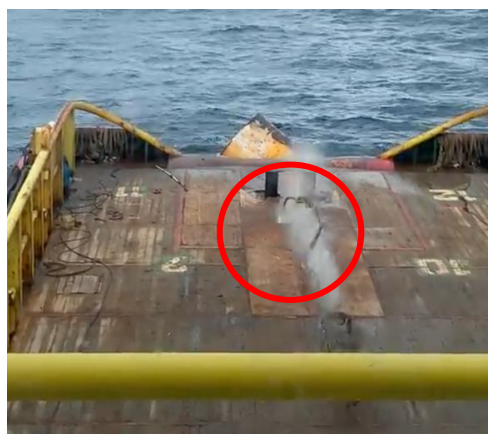
Figure 7 Buoy catcher breaks due to buoy getting caught so that the tension increases Source: Personal Documentation (2023)
