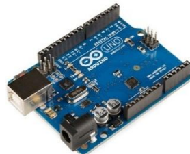
Figure 2. 2 Arduino Uno R3 Source : Wikipedia Bahasa Indonesia
