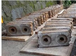
Figure 2. Left to Right: paving blocks mixed with plastic waste, crushed plastic bottle waste.
