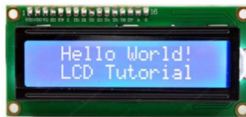
Figure 4. LCD 16x2 + I2C Source: Toughthware
