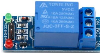
Figure 6. Relay 1 channel Source: Superbtech
