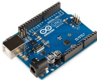
Figure 1. Arduino UNO R3 Source: Wikipedia Bahasa Indonesia
