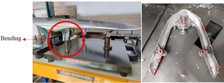
Figure 9 Examples of defects in products
