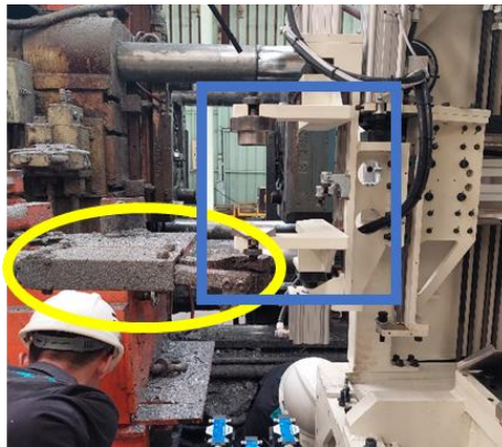
Figure 8 Casting machine gripper and trimming press
