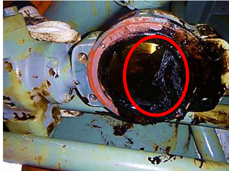
Figure 2. The presence of cotton wool on the valve
